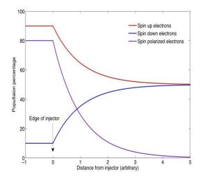
A plot showing a spin up, spin down and the resulting spin polarized population of electrons. Inside a spin injector, the polarization is constant, while outside the injector, the polarization decays exponentially to zero as the spin up and down populations go to equilibrium.
